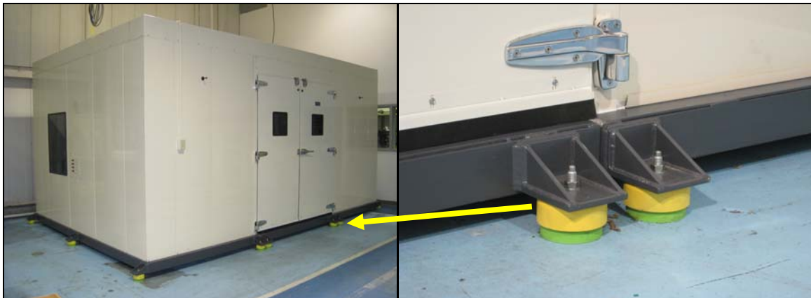
Acoustic Test Cell Floor Supports on AirLoc PRP Jacmounts
