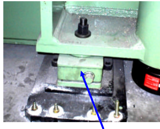
AirLoc Rigid Clamp® Wedgmound with Spherical Seat, Bolt-through Design
